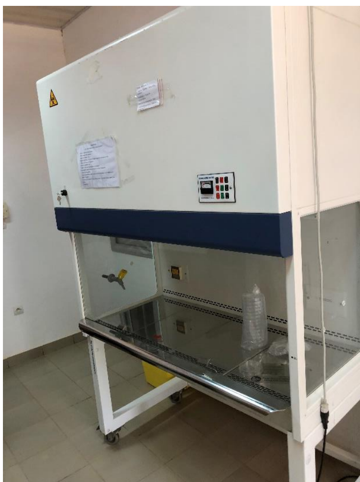
Figure 12. Non-functioning fume hood probably because of a dirty filter
