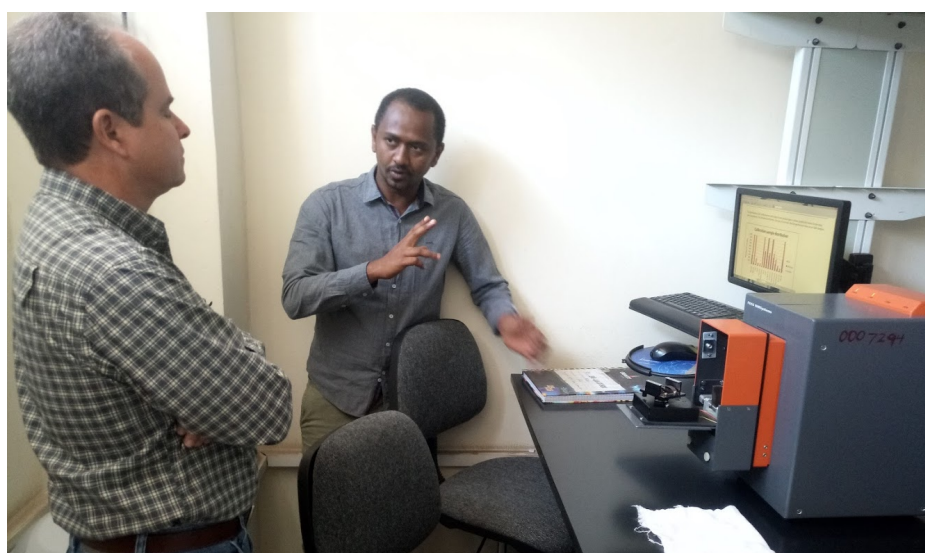
Discussing near-infrared spectroscopy (NIRS) in Ethiopia are Dr. Jose Dubeux, University of Florida, and Legesse Shiferaw, a lab technician from the Ethiopian Institute of Agricultural Research. This FOSS NIRS performs quick analyses of the nutritional values of large numbers of feed samples.
