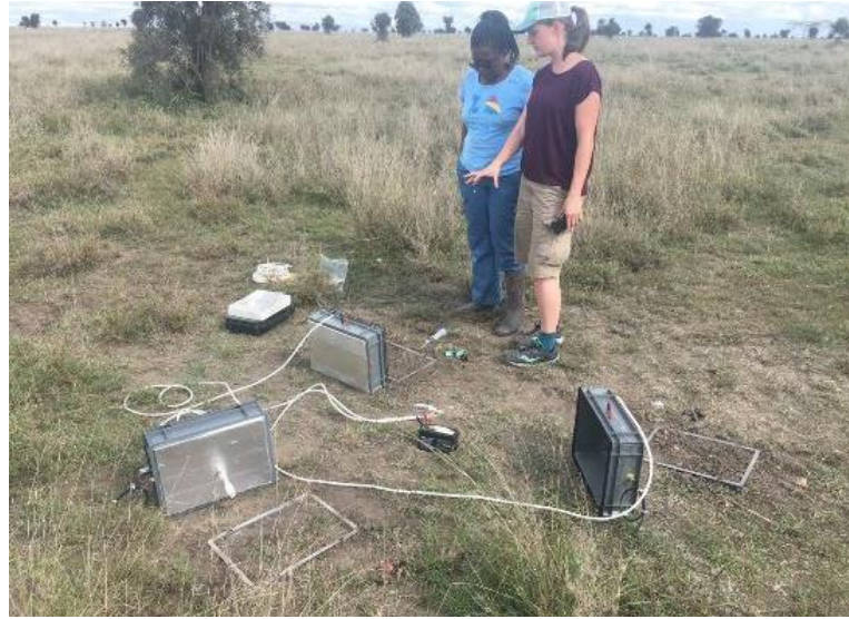
>300 manual chambers for field GHG measurements (with GC or Laser/IRGA)
