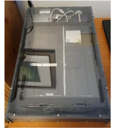
1 Root scanner in Eddy tower footprint (root growth dynamics)
