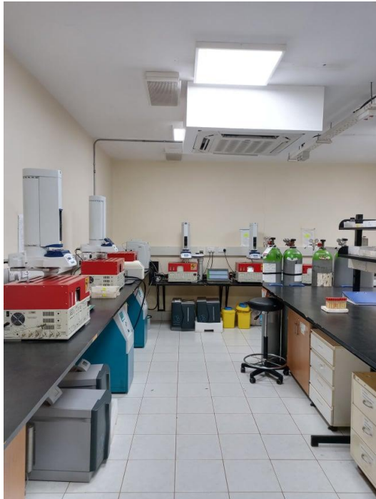
6 Gas Chromatographs ( N_2O , CH_4 , CO_2 ) ( SF_6 will be added)
