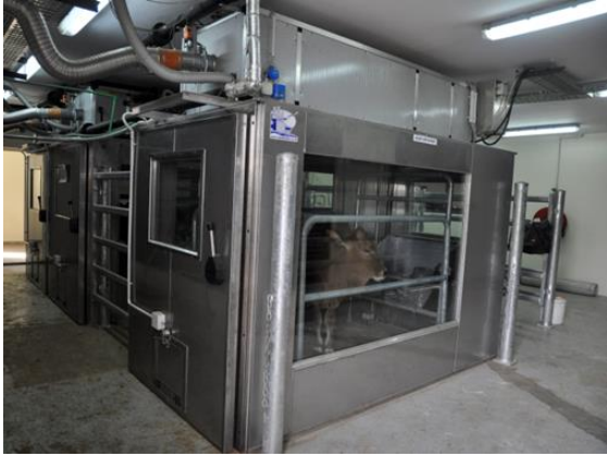
3 Large Ruminant Chambers
