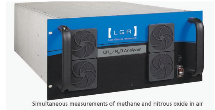
1 Los Gatos Research (LGR) Analyzer ( CH_4 and N_2O )
