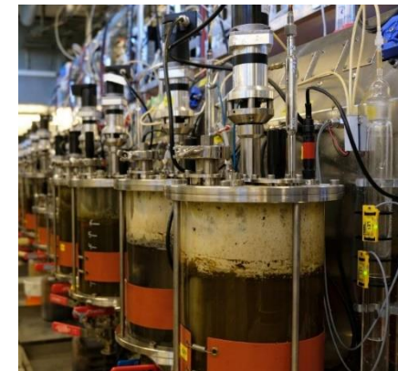
4 Continuously Stirred Tank Reactors (CSTR) (to be set up in 2023)
