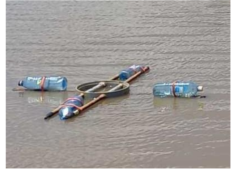
3 floating chambers for water GHG measurements
