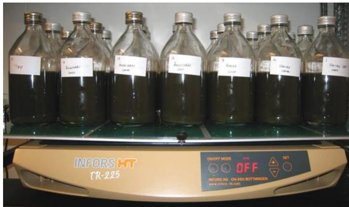
175 Anaerobic digestion/biogas batch bottles
