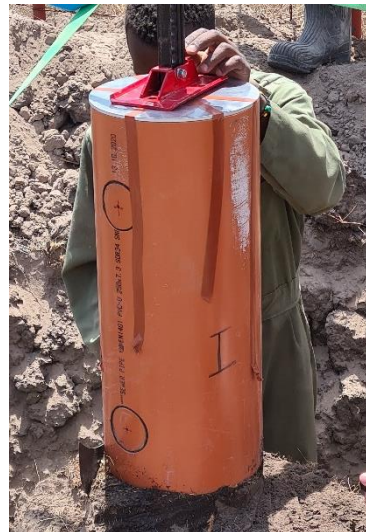
1 Lysimeter (evapotranspiration → drought stress)
