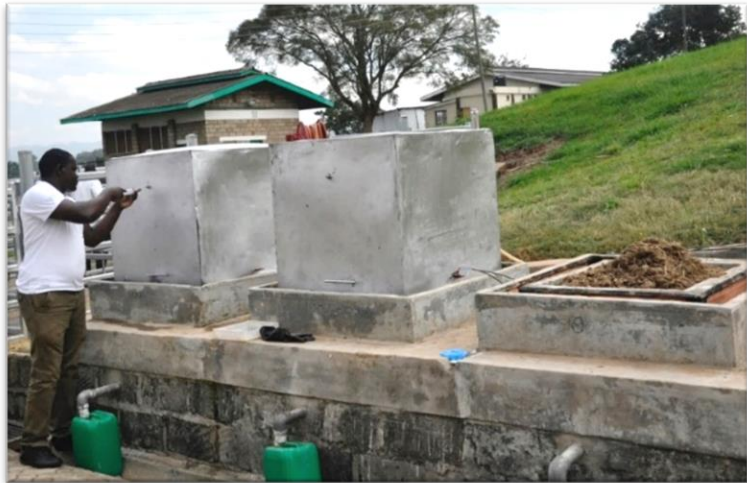
Chambers for manure heap measurements (9 with 100 kg capacity, 30 with 250 kg capacity)
