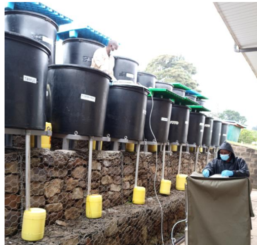
Chambers for manure heap measurements (9 with 100 kg capacity, 30 with 250 kg capacity)
