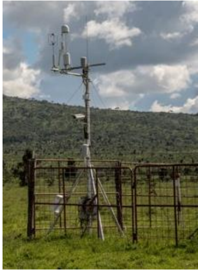
2 Eddy Covariance Flux Towers (CO 2 , H 2 O, CH 4 )
