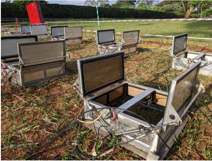
18 automatic soil GHG chambers + Picarro laser analyzer (soon to be deployed with mobile field lab)
